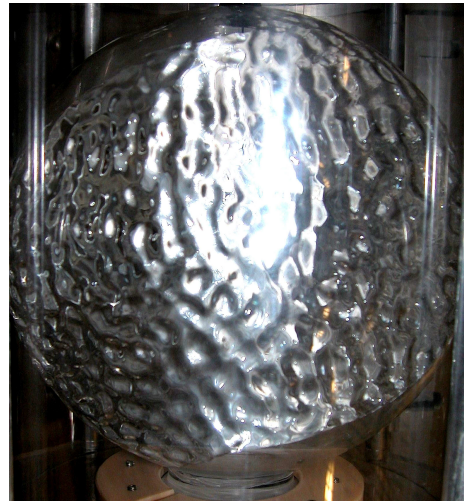
FIG. 3: Two-dimensional spherical subharmonic wave patterns under sinusoidal forcing at frequency 60 Hz. Spherical container filled with 20 cl of water.
