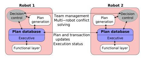
Fig. 1. In this architecture, each robot plan is managed by its own plan database. Parts of these plans are shared among databases. Decision control manages plan generation, team management and solves conflicts between execution and planning
