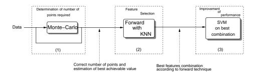
**Fig. 4.** Schematic view of the proposed methodology: (1) An appropriate number of data points to work with is determined using a Monte-Carlo method for statistical stability; (2) The forward selection is performed using a KNN classifier; (3) A good feature set is selected and performance is improved using SVM.
