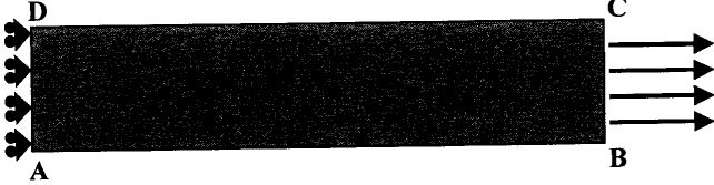
Fig. 4. Boundary conditions of the problem. On side AD, the displacements were fixed. On side BC, 5 m/s velocities were applied.
