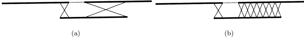
Fig. 5. (a) Transverse joint with one cross-rod. (b) Transverse joint using several cross-rods.
