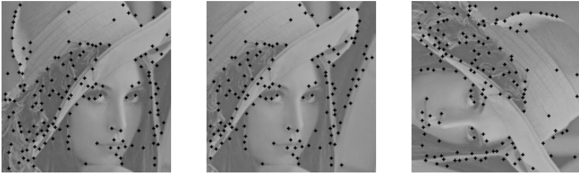
Figure 4. Points of interest using the Stephen-Harris detector, the detector is quite robust to translations and rotations.
