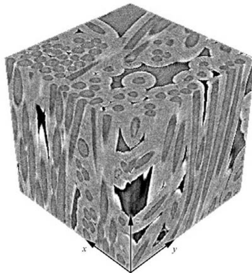
Fig. 1. A synchrotron microtomograph of a 0.0033 \text{ mm}^3 (side length < 0.15 \text{ mm} ) cubic sample of a C/C composite. Voxel size is 0.745 \mu\text{m} .
