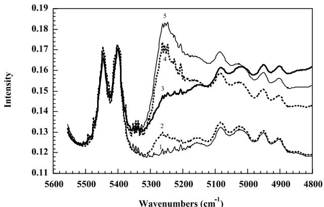
Fig. 8. Near-infrared spectra in the  $4800\text{--}5600\text{ cm}^{-1}$  range of pure PDMS (1) and of PDMS composites filled with 20 phr of silica: fumed silica of specific surface area of  $300\text{ m}^2\text{ g}^{-1}$  (2); in situ silica particles generated with the use of different catalysts: DEA (3); DBTDA (4); DBTDL (5).
