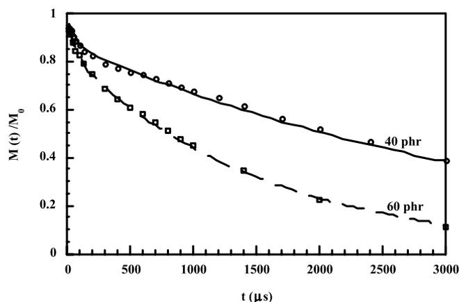
Fig. 11. Proton NMR relaxation data for tin-catalyzed PDMS/SiO<sub>2</sub> composites.
