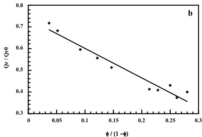
Fig. 9. Dependence of rubber phase swelling on the amount of filler (a) and plot of  $Q_r/Q_{r0}$  against filler loading expressed as volume ratio of filler to rubber (b).
