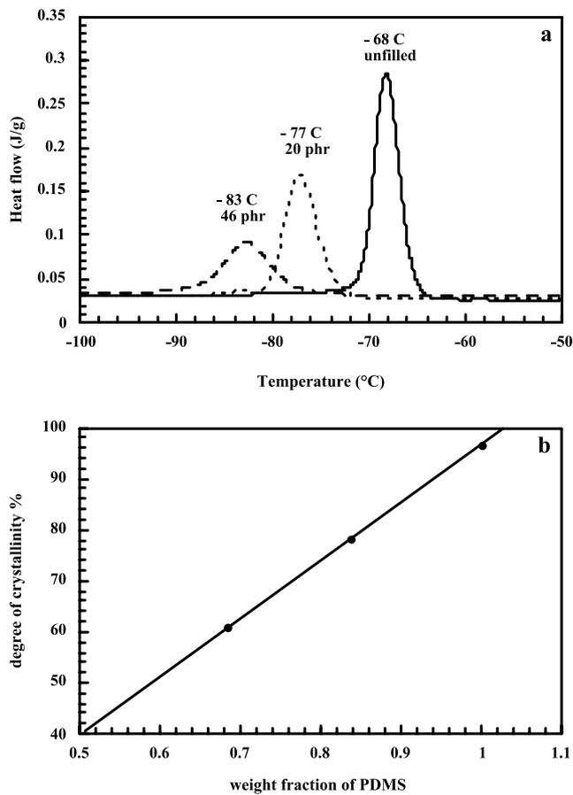
Fig. 10. Impact of the amount of filler (silica generated under DBTDL catalyst) on the crystallization peak (a) and on the degree of crystallinity (b).
