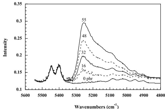
Fig. 6. Near-infrared spectra in the  $4800\text{--}5600\text{ cm}^{-1}$  range of pure PDMS and DBTDA-catalyzed PDMS/ $\text{SiO}_2$  composites: each curve is labelled with the amount of filler in phr (parts per hundred parts of rubber).
