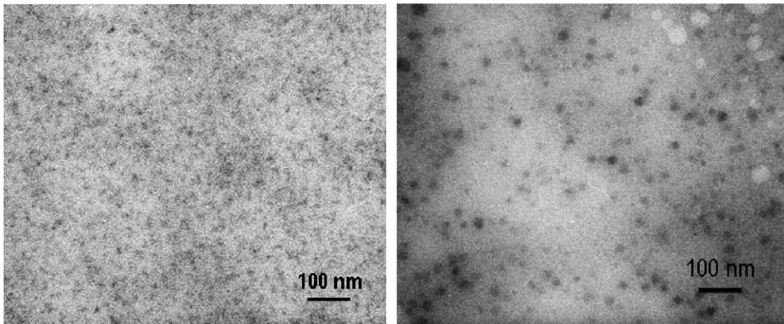
Fig. 1. TEM images of composites filled with 10 phr of SiO<sub>2</sub> precipitated into a PDMS network catalyzed by 3 wt% (DBTDL) (left) and by 3 wt% DEA (right).
