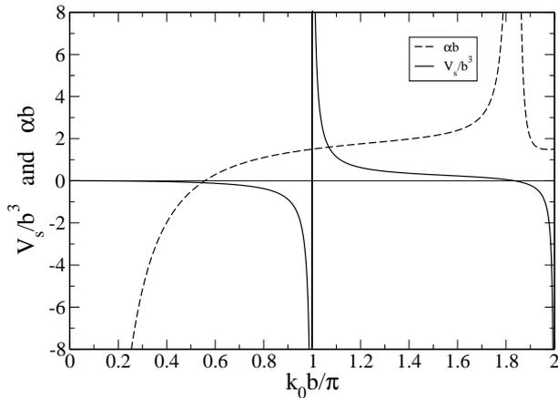
FIG. 1: For a square well interaction potential  $V(r) = -\frac{\hbar^2 k_0^2}{m} \theta(b-r)$ , where  $\theta$  is the Heaviside function, values of  $\alpha$  in units of  $1/b$  (dashed line) and  $\mathcal{V}_s$  in units of  $b^3$  (solid line) as functions of  $k_0 b$ . Note the divergence of  $\alpha$  when  $\mathcal{V}_s = 0$ .
