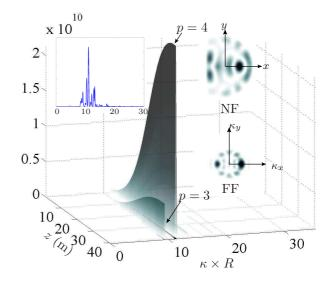
FIG. 2: Two-dimensional plot of  $C(\kappa; z)$  defined in (6) for  $L_z = 1.3 \,\mathrm{m}$ . Left inset: spectrum at z = 0. Right Inset: near-field (NF) and far-field (FF) intensities at the maximum signal amplification length  $z_{max} = 39 \,\mathrm{m}$ .
