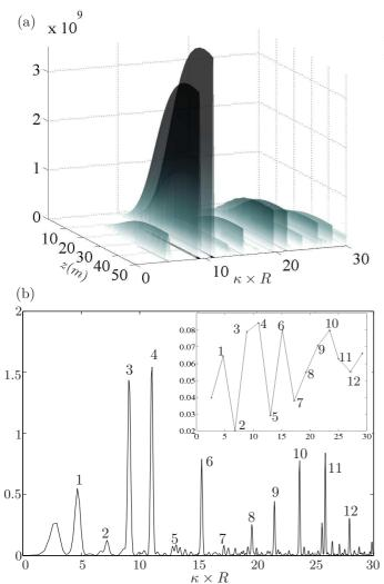
FIG. 3: (a) Evolution of  $C(\kappa;z)$  along the fiber for an incoherent initial illumination. (b) Instantaneous spectrum averaged over 5 different incoherent illuminations. The inset shows the overlap integral between the intensity of the calculated scar modes and the doped area.
