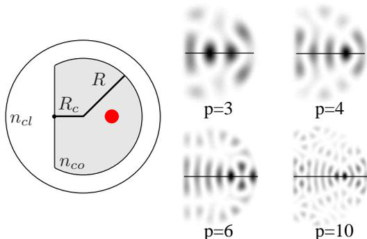
FIG. 1: Transverse cross section of the D-shaped multimode fiber and 4 scar modes associated to the shortest periodic orbit.
