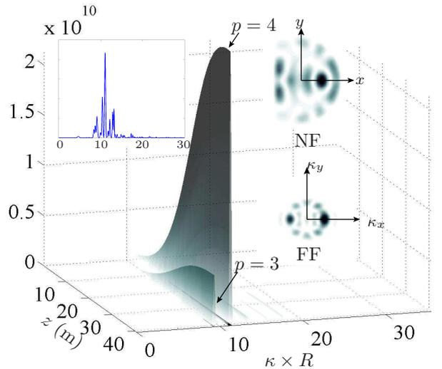
FIG. 2: Two-dimensional plot of  $C(\kappa; z)$  defined in (6) for  $L_z = 1.3$  m. Left inset: spectrum at  $z = 0$ . Right Inset: near-field (NF) and far-field (FF) intensities at the maximum signal amplification length  $z_{max} = 39$  m.
