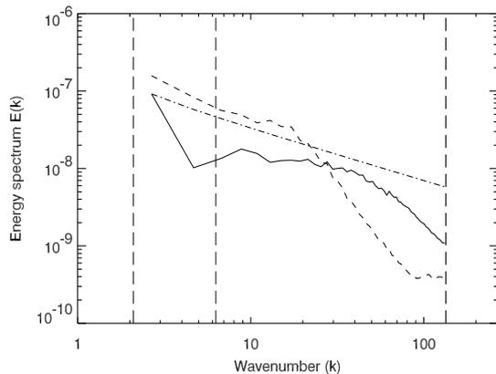
**Fig. 7.** Energy spectra of the magnetic energy density  $B^2/2\mu_0(k)$  (solid curve) and kinetic energy density  $\frac{1}{2}\rho u^2(k)$  (dashed curve) at time = 512 years, and a line corresponding to a power-law with an exponent of  $-2/3$  (dashed-dotted line). The vertical lines, from left to right, denote the wavenumbers corresponding to the computational box size  $k_0$ , the stellar radius  $k_R$ , and the Nyquist frequency  $k_{Ny}$  (the numerical resolution).
