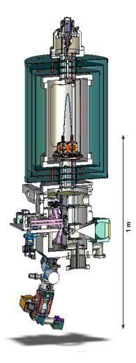
Fig. 1. Cut-away view of the FOCS-2 continuous cesium fountain clock showing the pre-source, the launch collimation and detection module, the parabolic flight of atoms thought the microwave cavity (Fig. 8) and the location of the velocity-selective light trap (Fig. 6).
