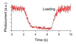
Fig. 3. Absorption of a probe laser beam along y by a static optical molasses in the FOCS-2 source as a function of time following interruption of the presource beams. Span=10 s. The loading time constant of about 1 s is compatible with a background pressure of  $<2\times10^{-9}$  mbar.
