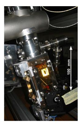
Fig. 2. Photo of the pre-source installed at the base of the FOCS-2 fountain adjacent to the ion pump(left). The gold-coated prisms used to relect the cris-cross laser beams are clearly visible. The cesium reservoir can be seen on the right of the image. The upper part shows the isolation valve beween pre-source and main fountain chamber.
