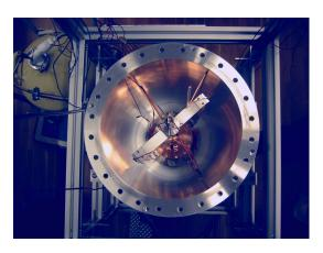
Fig. 8. Bird's eye view of the microwave cavity of FOCS-2 installed on its turntable in the vacuum chamber showing the cut-off tubes and the arms used to rotate the ensemble by exactly  $180^{\circ}$ .
