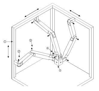
Figure 5: A fully isotropic parallel mechanism
