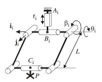
Figure 7: Legs kinematics of the Orthoglide
