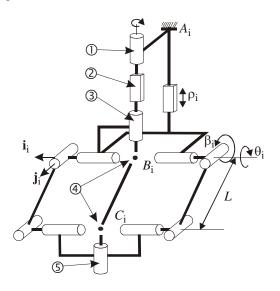
Figure 11: New design for the legs of the Orthoglide
