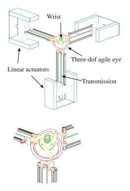
Figure 13: A six-dof haptic device 3T+3R
