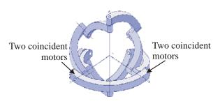
Figure 9: Redundant spherical wrist
