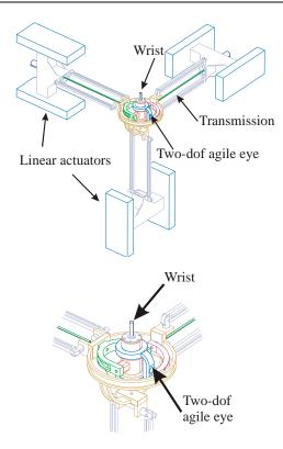
Figure 14: Six-dof haptic device 3T+2R+1R
