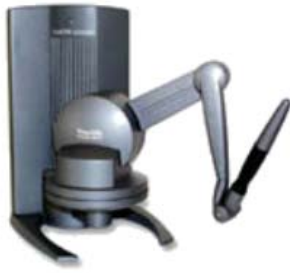
Figure 1: The Phantom Desktop provides one single point of contact to the user
