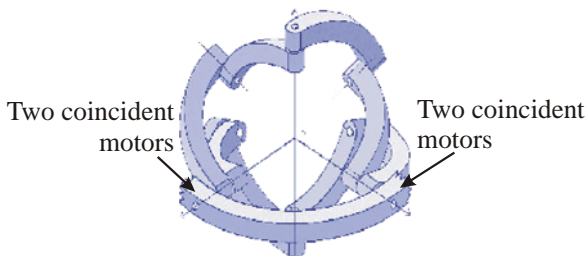
Figure 9: Redundant spherical wrist
