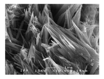
Fig. 14. SEM image of secondary electrons (× 10,000) of jaffeite.
