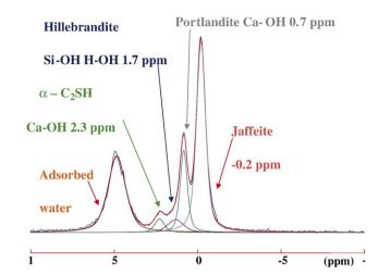
Fig. 16. <sup>1</sup>H-NMR CRAMPS spectrum of the  $C_3S$  hydrated sample at 200 °C under 600 bar for 14 days.
