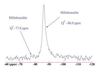
Fig. 3. <sup>29</sup>Si-NMR spectrum (SPE) of hillebrandite.
