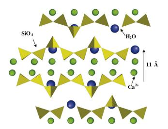
Fig. 5. Structure of C-S-H [20], courtesy of J.Minet.
