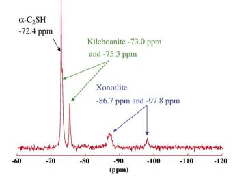
Fig. 19.  $^{29}$ Si-NMR spectrum (SPE) of the C<sub>3</sub>S hydrated sample at 200 °C under 600 bar for 4 days with silica addition.
