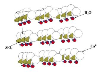
Fig. 7. Crystal structure of α-dicalcium silicate hydrate.
