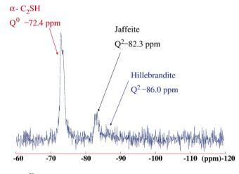
Fig. 15.  $^{29}\text{Si-NMR}$  spectrum (SPE) of the C3S hydrated sample at 200 °C under 600 bar for 14 days.
