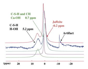
Fig. 11. <sup>1</sup>H-NMR CRAMPS spectrum of the  $C_3S$  hydrated sample at 120 °C under 400 bar for 4 days.
