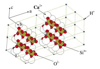
Fig. 8. Crystal structure of xonotlite.
