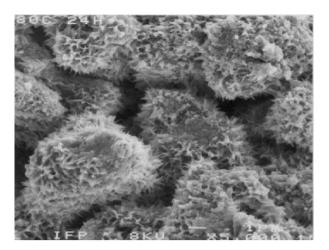
Fig. 12. SEM image of secondary electrons (× 5000) of the C-S-H.
