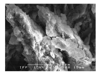
Fig. 18. SEM image of secondary electrons ( $\times$  3500) of  $\alpha\text{-dicalcium silicate}$  hydrate.
