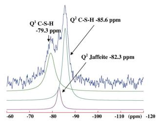
Fig. 10.  $^{29}$ Si-NMR spectrum (SPE) of the C<sub>3</sub>S hydrated sample at 120 °C under 400 bar for 4 days.
