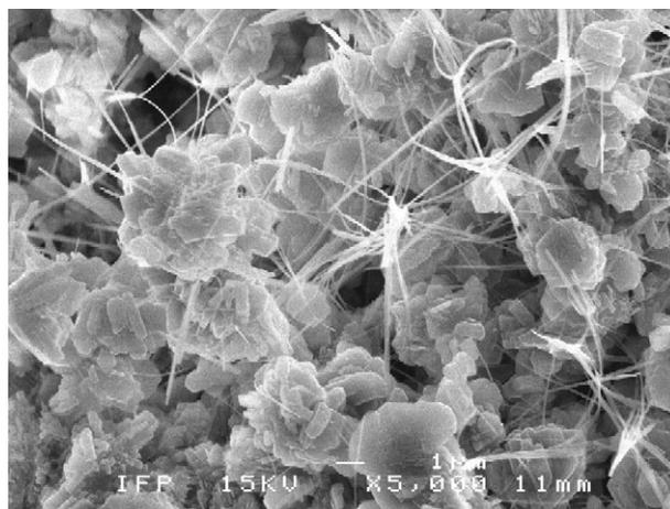
Fig. 20. SEM image of secondary electrons ( $\times 5000$ ) of xonotlite (fibres) and kilchoanite (globules).
