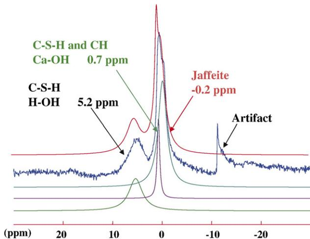
Fig. 11.  $^1\text{H}$ -NMR CRAMPS spectrum of the  $\text{C}_3\text{S}$  hydrated sample at  $120\text{ }^\circ\text{C}$  under 400 bar for 4 days.
