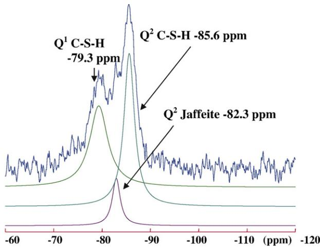
Fig. 10.  $^{29}\text{Si}$ -NMR spectrum (SPE) of the  $\text{C}_3\text{S}$  hydrated sample at  $120\text{ }^\circ\text{C}$  under 400 bar for 4 days.
