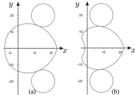
Fig. 9. Design strategies of Slide-o-Cam with (a)  $\phi_{cam} = 16\text{mm}$ ,  $a_4 = 7\text{mm}$ ,  $p = 40\text{mm}$ ,  $\mu_{max} = 53.8^\circ$  and  $\Delta\mu = 35.6^\circ$  and (b)  $\phi_{cam} = 3\text{mm}$ ,  $a_4 = 7\text{mm}$ ,  $p = 40\text{mm}$ ,  $\mu_{max} = 15.6^\circ$  and  $\Delta\mu = 11.1^\circ$
