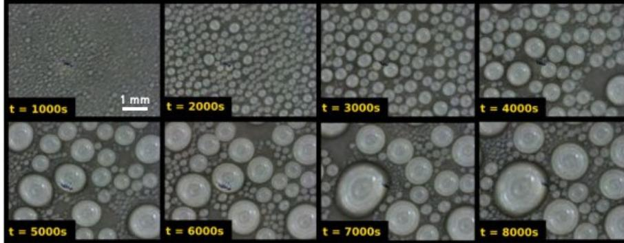
Figure 9: Visualization of the evolution of condensation obtained by radiative cooling on the surface C1 with  $T_a = 298.3$  K and  $RH = 95$  %. Size of the pictures :  $6.1 \times 4.6$  mm<sup>2</sup>.
