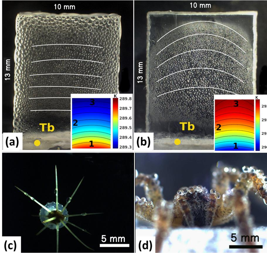
Figure 5: Top : PMMA block ( $10 \times 13 \times 8 \text{ mm}^3$ ) cooled by radiation (a) and conduction (b) from its base (temperature  $T_b$ ),  $t=5830 \text{ s}$  after the beginning of condensation with chamber conditions :  $T_1 = 295 \text{ K}$  ,  $\text{RH}=95 \%$  ,  $T_b = 289.8 \text{ K}$ . Bottom : condensation obtained by radiative cooling on cactus spines (c) and a spider (d). Inserts in a) and b) : simulated temperature distribution (see text for simulation details)
