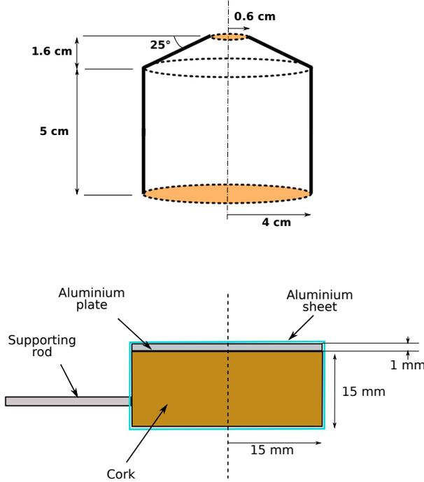
Figure 2: Top : Schematics of the mirrors (7), the colored zones corresponds to the openings to the outside. The interrupted line shows the axis of revolution. Bottom : Schematics of the sample holder (3). The interrupted line shows the axis of revolution.
