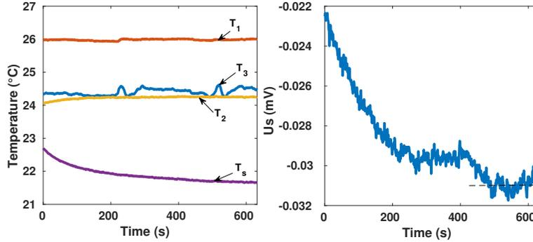
Figure 7: Temperatures of  $T_1$  : incoming air,  $T_2$  : mirrors,  $T_3$  :IR transparent window and  $T_s$  : sensor, during a radiative heat flux measurement.  $U_s$  : voltage measured by the radiative heat flux sensor.
