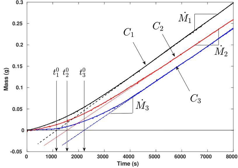
Figure 10: Evolution of the mass weighed by the balance during the condensation obtained by radiative cooling of surfaces (2) of different emissivities and contact angle : Surface C1 ( $\varepsilon_{C1} = 0.96$ ,  $\theta_{C1} = 84.6^\circ$ ), Surface C2 ( $\varepsilon_{C2} = 0.88$ ,  $\theta_{C2} = 65.9^\circ$ ), Surface C3 ( $\varepsilon_{C3} = 0.05$ ,  $\theta_{C3} = 65.9^\circ$ ). Chamber conditions are  $T_a = 298.3$  K and  $RH = 95\%$ .
