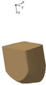
Fig. 7: Workspace defined as the set of points P in the fixed Cartesian frame R_b
