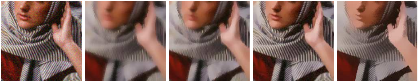
(a) Noisy image ( \sigma = 15 ). (b) p = 2 , local processing. (c) p = 1 , local processing. (d) p = 1 , nonlocal processing ( 3 \times 3 patch). (e) p = 1 , nonlocal processing ( 5 \times 5 patch).
