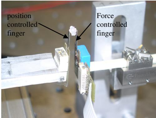
Figure 3: force controlled handling of a small component (size: 2mm)
