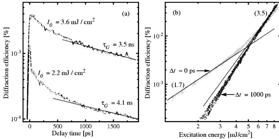
Fig. 4. Characteristics of light diffraction in ZnTe:V:Al at  $\lambda = 2.7 \mu\text{m}$ : (a) grating kinetics at various excitation energies and (b) dependencies of diffraction efficiency shown for different delay times of the probe beam. Numbers in the brackets indicate the characteristic EC slopes.
