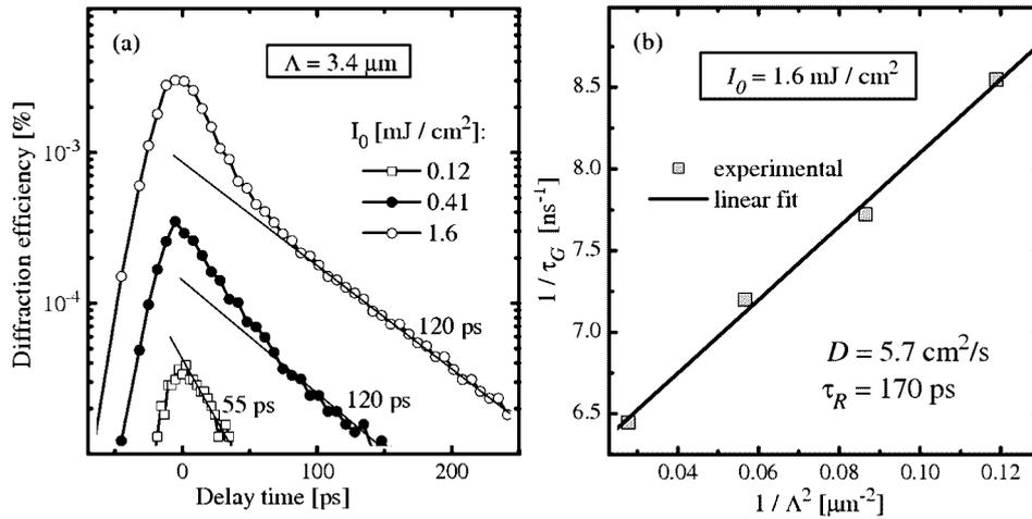
Fig. 3. Surface grating decay kinetics (a) and  $1/\tau_G \propto 1/\Lambda^2$  dependence (b) measured in ZnSe:Cr ( $N_{Cr} = 5 \times 10^{18} \text{ cm}^{-3}$ ) by using 355 nm wavelength light for the grating recording.
