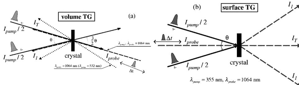
Fig. 1. Optical schemes for transient grating (TG) experiments: (a) volume gratings ( $hc/\lambda_{\text{pump}} < E_g$ ) with probe matched to the Bragg angle for  $\lambda_{\text{pump}} = \lambda_{\text{probe}}$  (dashed line) and  $\lambda_{\text{pump}} = \lambda_{\text{probe}}/2$  (dotted line) cases and (b) surface gratings ( $hc/\lambda_{\text{pump}} > E_g$ ).
