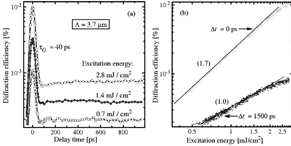
Fig. 2. Kinetics of FC grating decay (a) and exposure characteristics of diffraction efficiency (b) measured in ZnSe:Cr ( $N_{Cr} = 5 \times 10^{19} \text{ cm}^{-3}$ ) by using 534 nm wavelength light for the grating recording. Numbers in the brackets indicate the characteristic EC slopes.
