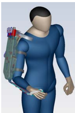
Fig. 2 Portable haptic device that will be integrated into our framework
