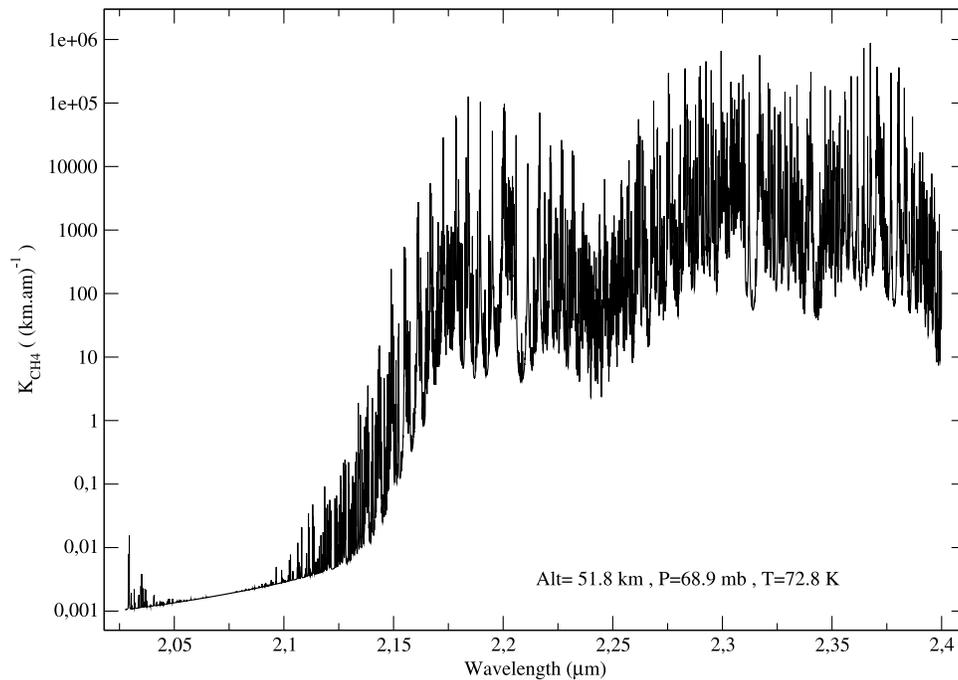
**Figure 3.** Example of the methane absorption coefficients used in the model. The ones shown were computed for a temperature of 72.8 K and a pressure of 68.9 mbar, which corresponds to an altitude of 51.8 km in Titan’s atmosphere.
