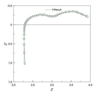
Figure 2 : Typical complex impedance spectrum of the cell recorded at 700°C under open circuit conditions.
