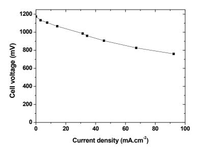
Figure 1 : Current voltage behaviour of  $Nd_{1.95}NiO_{4+\delta}$  cathode single cell operated at 700°C (with 30mL.min<sup>-1</sup> H<sub>2</sub> and 70mL.min<sup>-1</sup> air).
