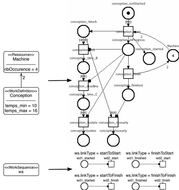
Figure 5: Translation schema from SIMPLEPDL to PetriNet
