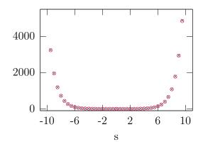
Figure 3. Plot of the large deviation function  $\frac{1}{L}\psi_Q(s)$  of the Asymmetric Simple Exclusion Process, for L = 400 sites and N = 200 particles. The jump rates are p = 1.2 and q = 0.8, whence  $E \simeq -0.2$ . Blue crosses and red circles correspond to direct computation and thermodynamic integration respectively. The asymmetry appears when comparing the extreme points  $s = \pm 9.5$ .
