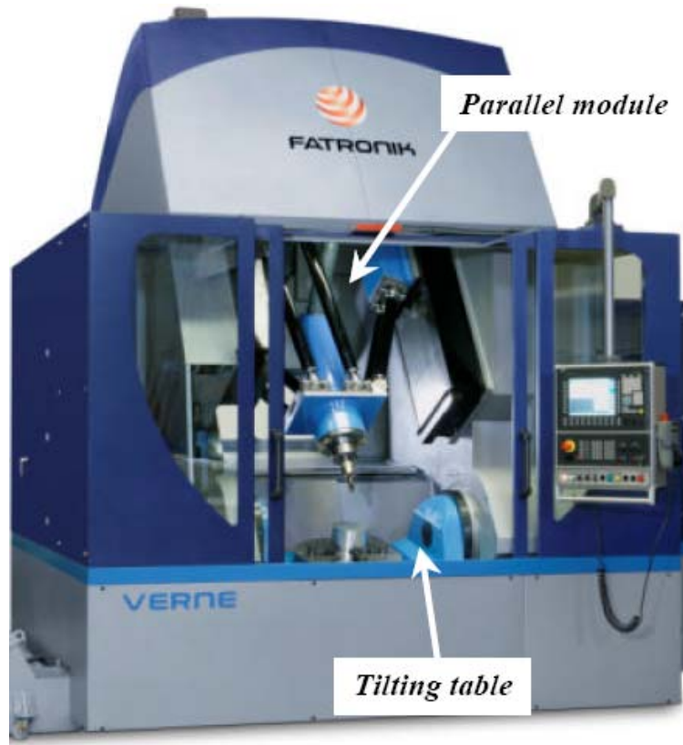
Figure 1: Overall View of the VERNE Machine
