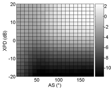
Fig. 3: Difference between the triple-polarized and the single-polarized channel capacity of  $4 \times 4$  MIMO systems in the functions of XPD and AS
