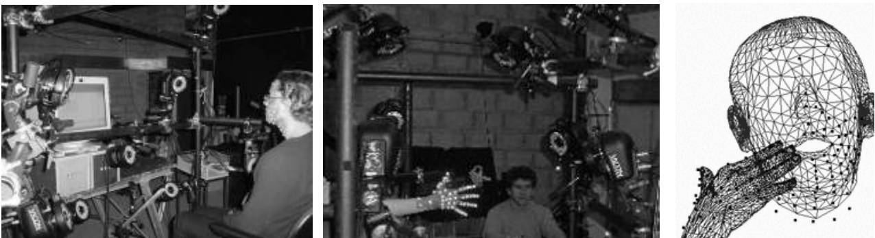
Figure 3. Capturing and cloning face and hand movements of a human cueer. Left and centre: the experimental settings. Right: the resulting shape model used to animate the virtual speech cueer.
