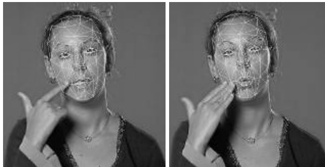
Figure 7. Tracking gestures using an adapted 3D face model with partial occlusions by the hand.
