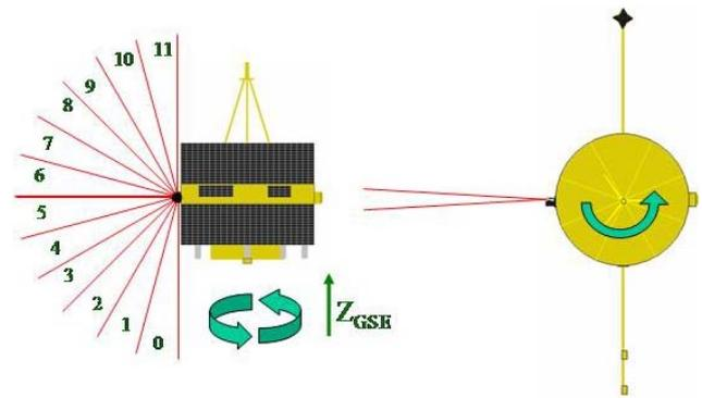
**Fig. 2.** Illustration of instantaneous field of view of a Double Star PEACE sensor. Left: Side view of spacecraft, spin axis points close to  $Z_{GSE}$ , the “look” directions from which electrons arrive to be measured by the 12 anodes are indicated. Right: Top view of spacecraft, showing instantaneous field of view (elevation acceptance angle) also illustrating configuration of magnetometer booms (note that on TC-1 the STAFF boom is not deployed).
