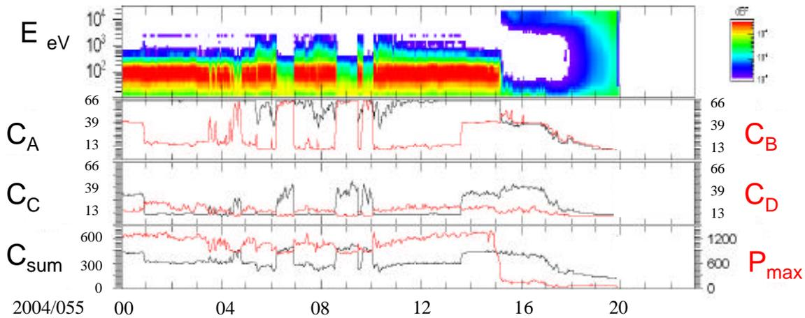
**Fig. 12.** Illustration of the variation with plasma environment of the number of transmitted JPEG coefficients per image.
