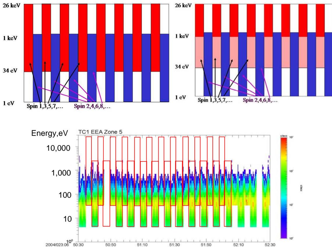
**Fig. 11.** (a) illustration of alternating preset mode; (b) illustration of option of returning only non-overlapping energy data from first sweep in a pair; (c) data plot showing coverage when operating as in mode outlined in (a).
