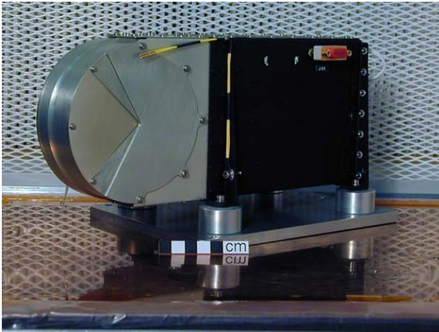
**Fig. 5.** A view of the TC-1 PEACE Sensor. Note the analyser head radiation shield material intended to protect the MCP, in particular the pie-slice plates and the enhanced thickness rim of the cylinder towards the aperture side of the sensor head.
