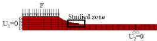
figure 1: Test specimen and boundary condition
