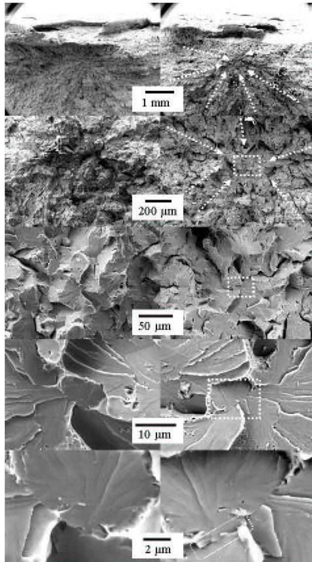
Figure 1: Identification of a triggering site (CVN #73 tested at  $-40^{\circ}\text{C}$ ). Example of the different steps used for the identification. On the matching surface photographs, dotted arrows were drawn to underline the macroscopic river patterns. Afterwards, boxes with dashed line were used to indicate the interest zone. On the last photograph, the triggering site, which is a grain boundary, is indicated by a dashed rectangle.
