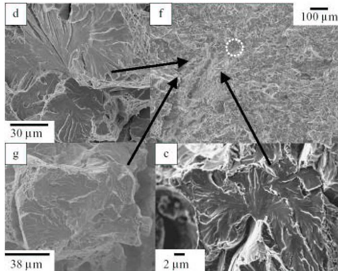
Figure 3: NT<sub>1,2</sub> #7 tested at  $-70^{\circ}\text{C}$ . Arrows locate the final micrographs taken by participants around the inclusion stringer. The circled zone drawn shows one potential triggering main site.
