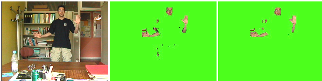
Fig. 4 . From left to right: original image, skin detection in the H and CbCr colour spaces.
