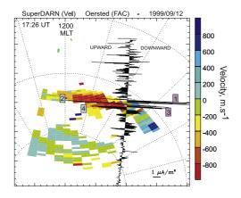
**Figure 3.** L-o-s velocity map (magnetic coordinates) of the Kapuskasing radar at 17:26 UT. The Ørsted orbit is superimposed on the map with the FAC intensities plotted perpendicular to the orbit. Labels (1) to (4) correspond to the four small-scale current sheets.
