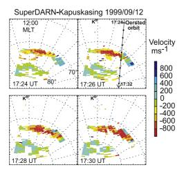
**Figure 1.** L-o-s velocity maps (magnetic coordinates) of the Kapuskasing (K) radar for the period 17:24–17:30 UT. Negative velocities represent motion away from the radar (colour-coded from yellow to red). The Ørsted orbit is superimposed on the 17:26 UT map (black dots are separated by one minute).
