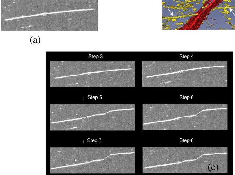
**Figure 4.** A natural vein-shaped inclusion in specimen ESTSYN01: (a) CT image in a vertical plane before loading (step 1), (b) 3D reconstruction after unloading (step 8), and (c) CT image in a vertical plane at different steps of loading
