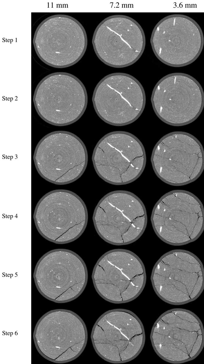
**Figure 5.** *Horizontal CT slices of specimen ESTSYN02 at different steps and for three different elevations*
