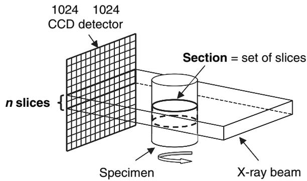
**Figure 3:** X-ray beam through the specimen to the phosphor screen
