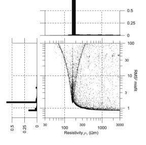
**Fig. 4.** Projection of all RMS<sup>2</sup> misfits *versus* the resistivity of the top layer obtained in the course of 20 CRS6 runs applied to the COPROD1 (DSII) data set with 3-layer test models. Along the axes, the corresponding histograms of the RMS<sup>2</sup> and  $\rho_1$  values are shown.
