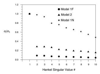
FIG. 10. A plot of  $\sigma_i/\sigma_1$  for the first 10 members (i = 1, ..., 10) of the Hankel singular value spectrum from each model using an annual mean basic state.
