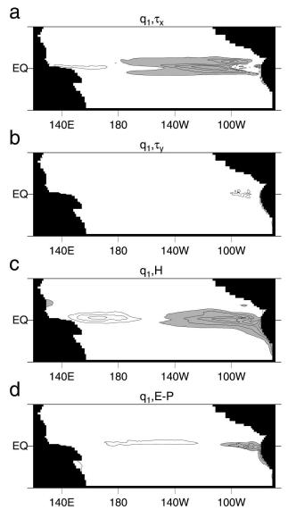
FIG. 2. The spatial structure of wind stress  $(\tau_x, \tau_y)$ , surface heat flux *H* and surface freshwater flux (E - P) for  $\mathbf{q}_1$  for model 1F and an annual mean basic state. In each case the contour interval is arbitrary, and shaded and unshaded regions are of opposite sign.
