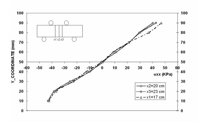
Figure 13: Numerical stress curves across medium section at different load (during the test)
