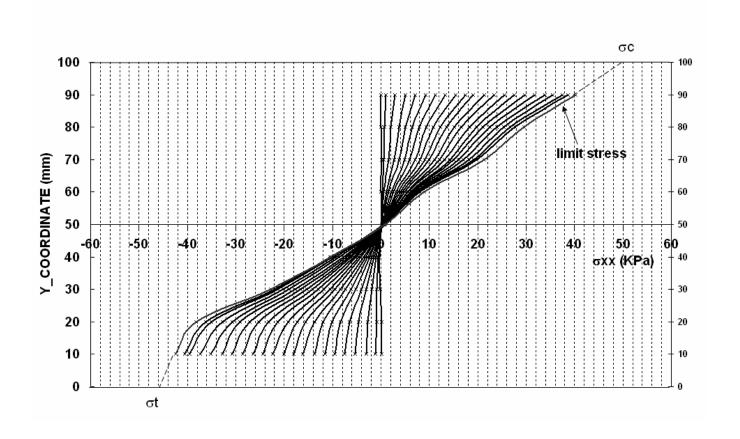
Figure14: Shape of stress diagram for differential method (Ajaz and Parry, 1975)
