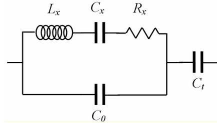
Figure 5. Electrical model of a crystal resonator whose motional parameters are  $L_x$ ,  $C_x$  and  $R_x$ .  $C_0$  is its parallel capacitor whereas  $C_t$  denotes the tuning series capacitor added to pull-up the overall resonant frequency.
