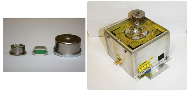
Figure 4. On left: various resonator cases (HC40, HC12, 5 MHz BVA). On right: the lower part of one resonator oven whose HC40 housing is visibly smaller than the 5 MHz BVA enclosure lied aside.
