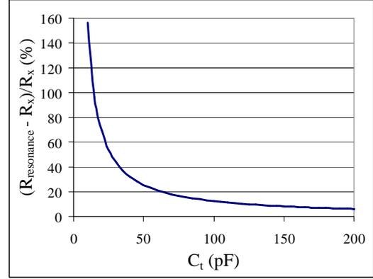
Figure 8. An example of the relative change of  $R_{resonance}$  versus  $C_t$ . One easily understands that the more the fluctuations of  $C_t$  the more the implied fluctuations of  $R_{resonance}$ .
