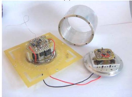
Figure 4. Double quartz crystal ovens.
