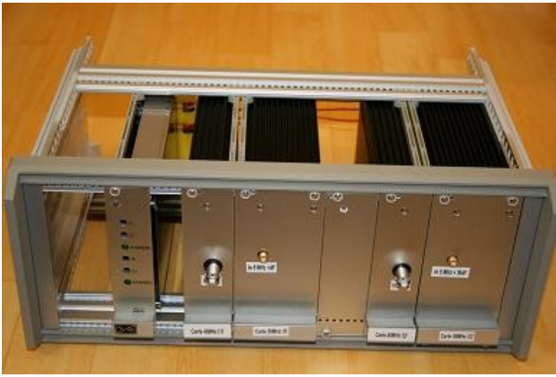
Figure 9: picture of the realized pre-multiplier
