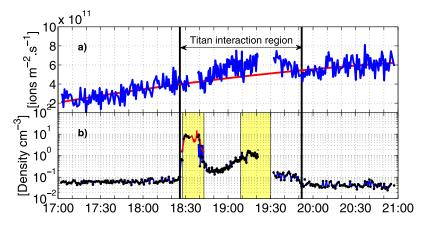
**Figure 4.** Plasma characteristics during the T9 encounter. (a) The ion flux directly measured by the Langmuir Probe sensor. (b) The electron number density derived from the upper hybrid resonance frequency (red) combined with the Langmuir Probe observations. The shaded area emphasizes the two main regions.
