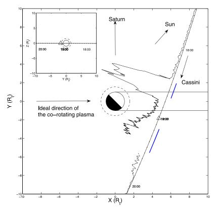
**Figure 1.** The T9 flyby trajectory in the Titan centered coordinate system (TIIS [cf *Backes et al.*, 2005]). Tickmarks on the trajectory are displayed every 5 minutes. The electron number density is projected along the trajectory of the spacecraft and emphasized the asymmetry of the plasma wake of Titan. The two blue lines indicate the time interval of the two main structures.
