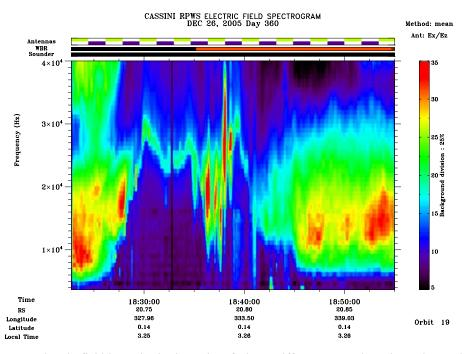
**Figure 2.** Plasma wave electric field intensity in the wake of Titan. Different waves have been detected and among them the upper hybrid resonance emissions between 10 kHz and 32 kHz.
