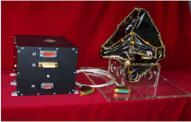
Fig. 1. The picture of the search coil and the electronic box of LFEW/TC-2.
