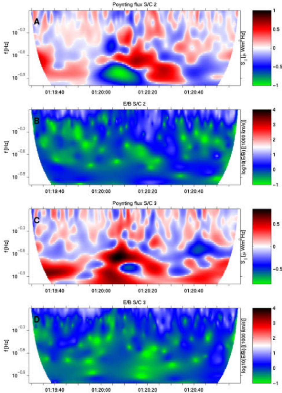
**Fig. 9.** Morelet wavelet analyses of the Poynting flux from Cluster satellites 2 and 3 (panels 1 and 3), where red (green) indicates downward (upward) flux, and the corresponding ratio of the electric and magnetic fields (panels 2 and 4). These results are obtained from data in panels (C) and (D) in Figs. 1 and 2. The observations indicate a mixture of downgoing and upgoing Alfvén waves.
