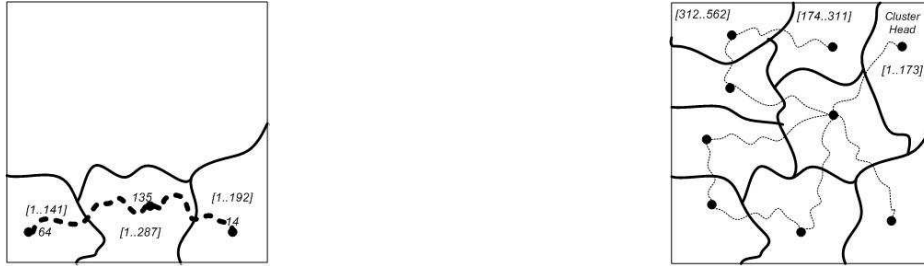
Figure 8. After the paths construction between clusters (dashed lines), the global initialization is just executed by means of the gossiping algorithm performed via these paths.
