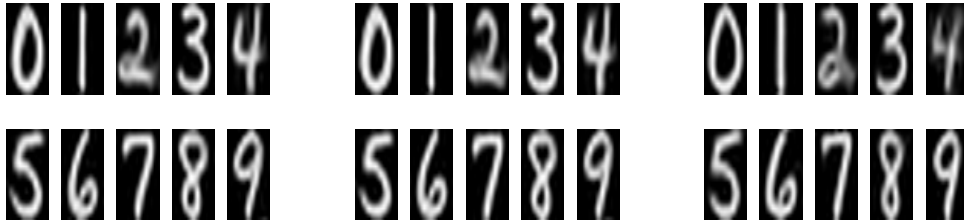
FIG. 5.5. Templates estimated with randomly chosen samples from the whole USPS database. Each image is one run of the algorithm with same initial conditions but different training sets of 20 images per digit each. The variability of the results is related to the huge variability inside the USPS database.
