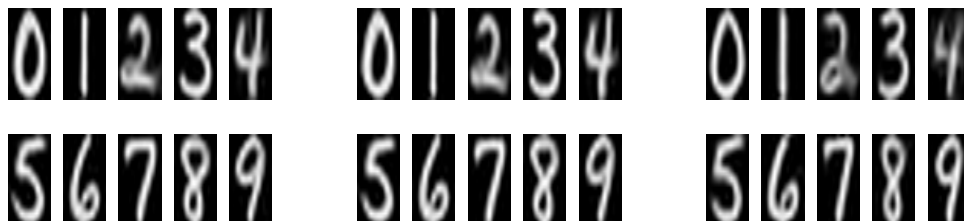
FIG. 5.5. Templates estimated with randomly chosen samples from the whole USPS database. Each image is one run of the algorithm with same initial conditions but different training sets of 20 images per digit each. The variability of the results is related to the huge variability inside the USPS database.
