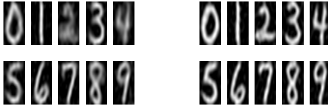
FIG. 4.9. Estimated prototypes in a noisy setting \sigma^2 = 1 : Left: with the mode approximation algorithm. Right: with the SAEM-MCMC coupling procedure.
